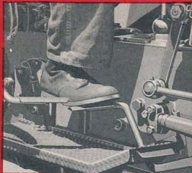
New duo-servo brakes operate together or separately through newly designed pedals, using right foot only, left foot remains free for clutch.
